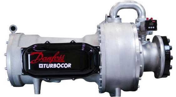
Based on proven TT series compressor technology, the VTT models are oil-free, variable-speed, magnetic bearing centrifugal compressors. They extend the stable operating envelope while simultaneously improving both full- and part-load efficiency. The VTT series of compressors is the first to introduce IntraFlow™ technology, an innovative and patent pending technology for improving compressor efficiency and providing an extended stable operating range while simplifying capacity control.
