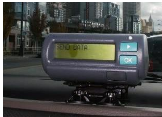
Figure 16. On-board unit for electronic road pricing. (Photo courtesy of the U.S. Department of Transportation)
