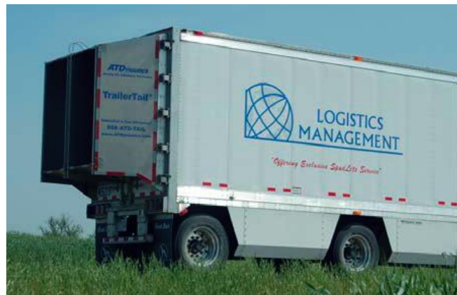
Figure 40. Side skirts and rear drag device added to a truck. (Photo: Rocky Mountain Institute)
