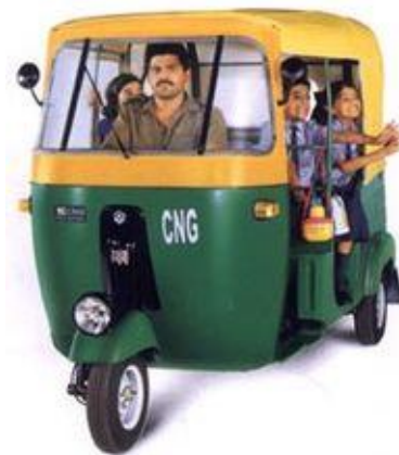
Figure 7. Three-wheel Bajaj rickshaw with a two-stroke engine powered by compressed natural gas. (Photo: www.dinesh.com )
