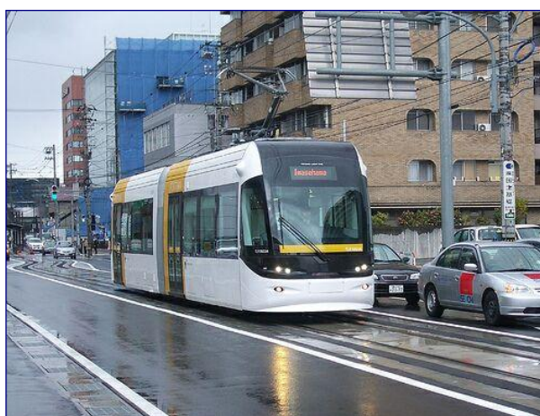
Figure 34. Street car portion of the tram-train Toyama commuter system. (Photo: Tsuda, Light Rail Now! )
