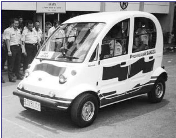
Figure 6. Four-wheel, four-stroke kancil in Indonesia, a cleaner alternative to the two-stroke gasoline- or diesel-powered bajaj . (Photo: www.treehugger.com )
